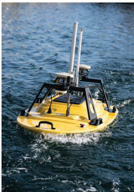
» Teledyne's 1800 and 1250 USVs support a wide variety of sensor packages optimized to survey, inspect, and monitor. (Photo credit: Teledyne Marine)
